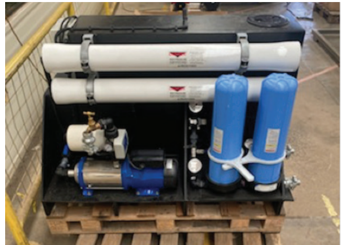
Nano Filtration Plant for washdown water.
